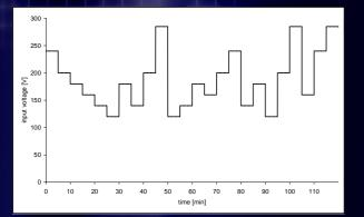
Voltage signal produced by the controller
